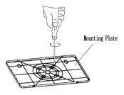
3.Securely attach mounting plate to J-box (not provided).
